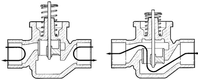
Fig. 1. Fluid flow through 2-way VC valve
