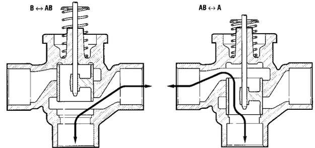
Fig. 2. Fluid flow through 3-way VC valve
